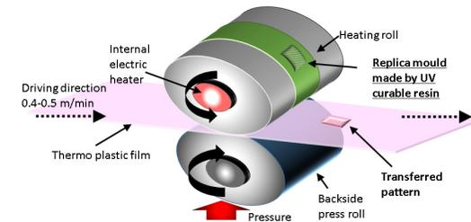
Figure 2. Schematic view of our T-R2RNIL equipment. The imprinting load was set to 800 N and the process temperature was raised up to 138 °C.
