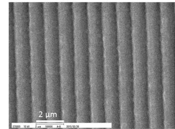
Figure 4. T-R2RNIL pattern at 138 °C on polymethylmethacrylate (PMMA) film.
