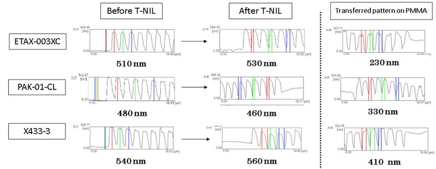
Figure 1. The pattern heights of the fabricated moulds before and after the planar T-NIL process, and the obtained PMMA patterns. The T-NIL conditions were 715 N for 1cm<sup>2</sup>, 120 °C for 5 min. The pattern height of PMMA using the replica mould made by X433-3 produced the sufficient height.
